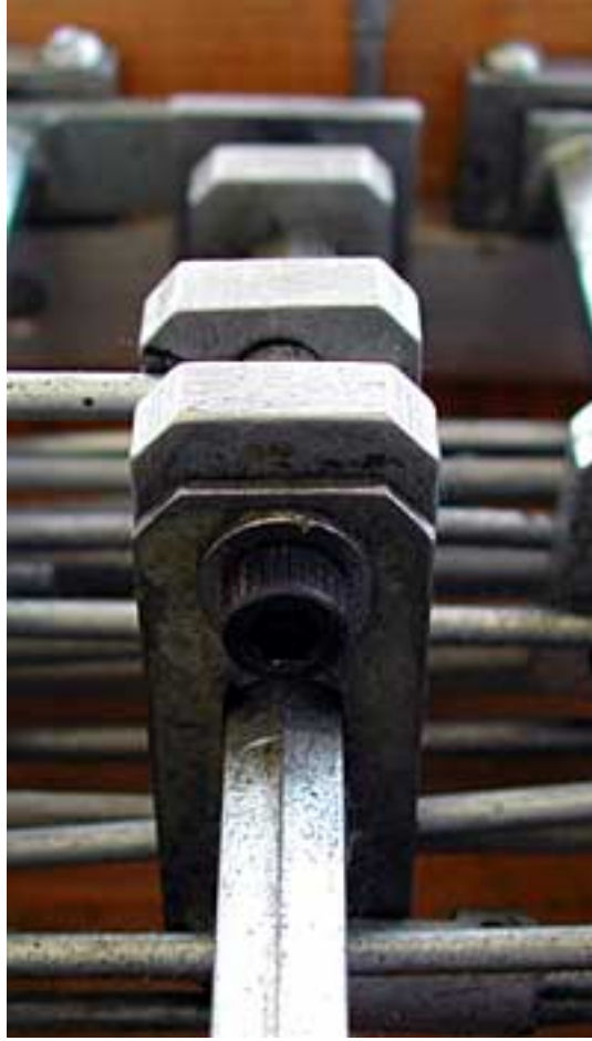
The adjustable single pull crank.
