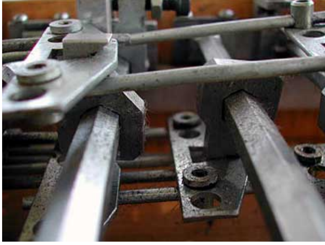
The hexagonal crossrods with bellcranks and yokes.
