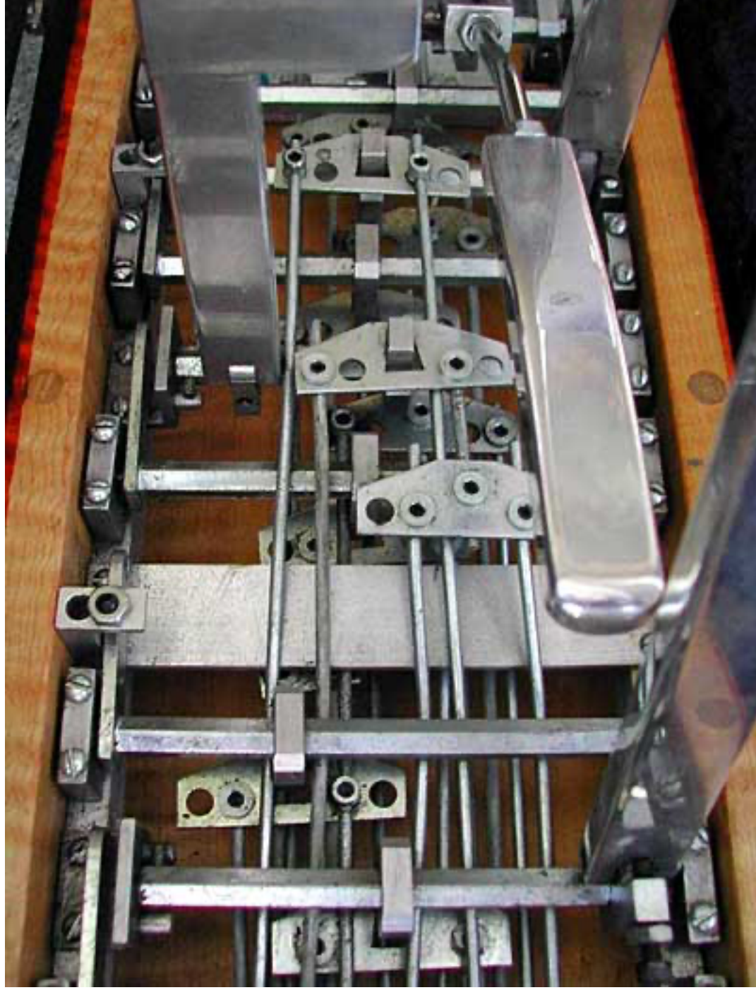
The plate across the body prevents the sides from spreading. Above the plate, on the left is one of the two pedal stops I have on it just to prevent any mushiness of that pedal. Note the vertical knee lever.
